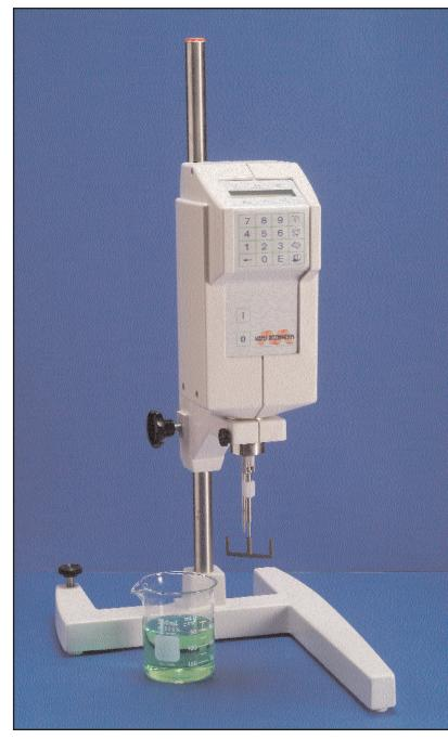
• Versatility: The design of the RM180 allows measurements to be made on a sample in any container. While attached to the viscometer, the open end of the measuring tube is immersed into the sample no matter what container the sample is in. • Keypad operation: A Liquid Crystal Display allows for clear instruction to prompt the user for input parameters. Keypad symbols allow for easy connection to a Personal Computer and calibration function.
