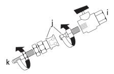
**NOTE:** EMD Millipore Corporation recommends using quick-disconnect fittings (j) between the ball valve and the hose connectors to facilitate attachment to and detachment from the vessel.
