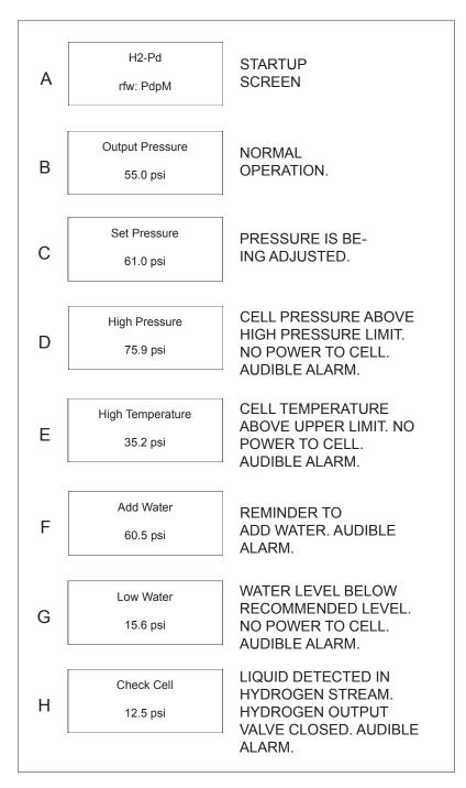
Figure 3 - Front Panel Display
