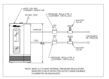
Figure 5- Recommended Installation
