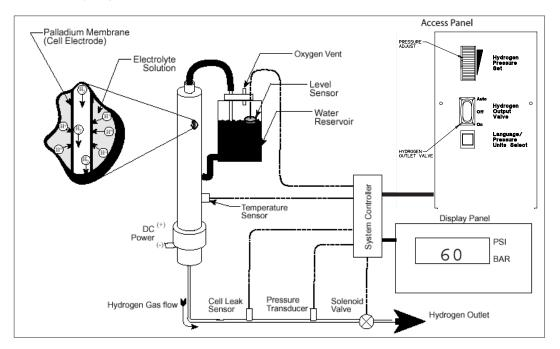
Figure 2 - Flow Schematic
