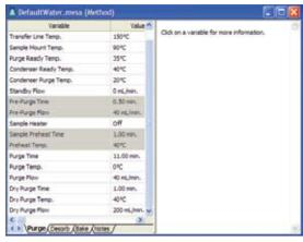
**Method Development Screen** - The Stratum TekLink<sup>TM</sup> Software comes pre-installed with methods for most applications. You can select one of these methods or if your application calls for a unique requirements, a customized method can be created to meet your analytical requirements for sample processing.
