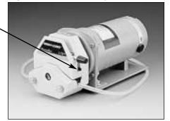
**NOTE:** There are a few combinations of tubing and materials that may require a further adjustment of the tubing retainers if the tubing creeps. Open pump head, move tubing retainer down one (1) notch, then close pump head. Turn pump on. If tubing creep persists, repeat procedure.
