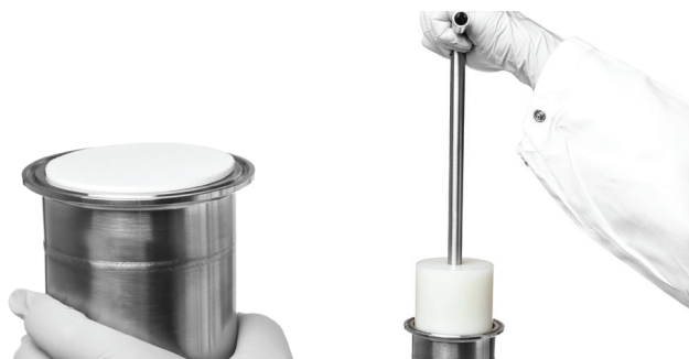
Figure 23. Inserting a frit into the SIM 2000 body using its frit insertion tool. Note that the insertion tool for SIM 500 and SIM 1000 does not have a handle.
