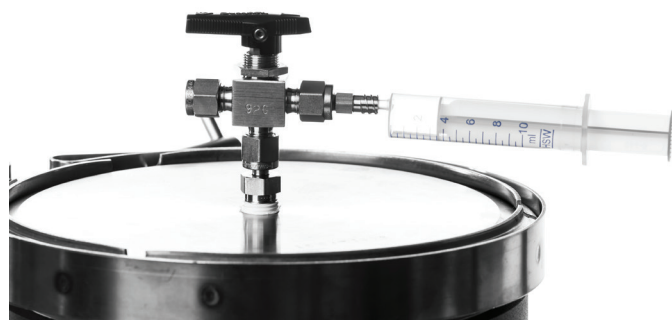
Figure 21. Alternatively, if the sample is soluble in a small volume of solvent, it can be injected with a syringe through a Luer-lock injection port on the radial compression module.
