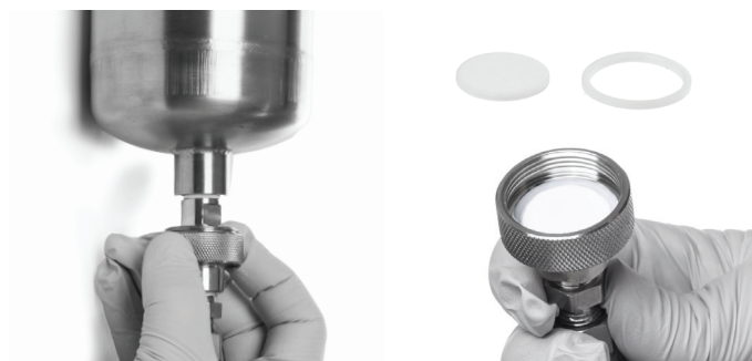
Figure 22. Inserting a bottom frit into the lower half of the frit holder.
