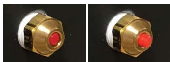
Figure 2. The pressure indicator sticks out when the pressure inside the radial compression module is more than 20 psi (1.4 bar).
