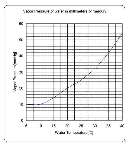
The above graph shows that vacuuming fluctuation is depending on water temperature in the bath.
