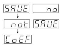
Step 5: Terminate configuration mode as describe in Configuration Mode.
