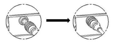
(3) When you connect with temperature probe, the LED lamp is automatically turned on.
