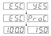
Temperature Probe Control Mode Connect temperature probe to the unit. The default mode will be automatically changed to the Temperature Probe Control Mode and display shows the temperature value detected by the probe.
