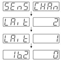
(4) In case of separating temperature probe from main body, the temperature display windows are showed follow message;
