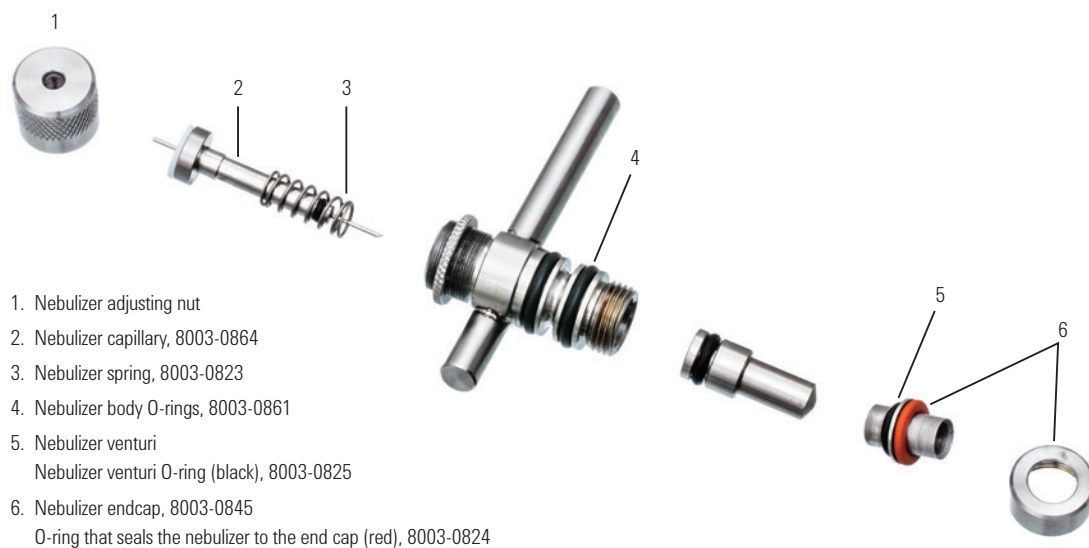
Exploded view of Nebulizer assembly, 8003-0828
