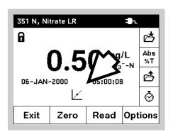
The Standard Adjust icon will appear on the measurement screen when Standard Adjust is enabled.
