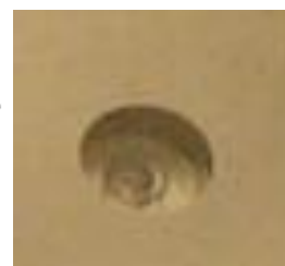
air bubble in the middle of the site glass
