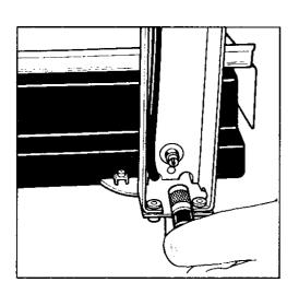
At the point of use, plug the cord of the power supply into the power receptacle(14) of the scale.
