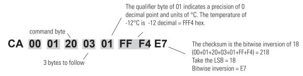
The master sets parameters in the chiller by sending one of the Set Functions as shown in Table 1. The master does not send a qualifier byte in the data field. The master should be preprogrammed to send the correct precision and units (it could also read the parameter of interest first to decode the correct precision and units needed).
