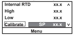
**5**. Press and enter the desired calibration temperature .
