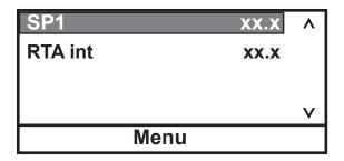
If this temperature on the Start/Status Displaysdoes not accurately reflect the actual temperature in the reservoir, an RTA can be applied. The RTA can be set  $\pm 10$ °C ( $\pm 18$ °F).
