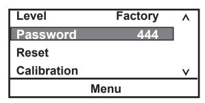
**NOTE** The controller resets to the **User** mode whenever the unit is turned off. The controller also resets to the **User** mode whenever the Start/Status Display is displayed continuously for 10 minutes.
