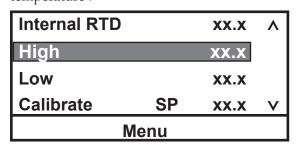
**6.** Highlight **Calibrate** and the press complete the procedure.
