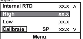
4. Highlight the **SP** temperature box and enter either the desired high or low setpoint value.
